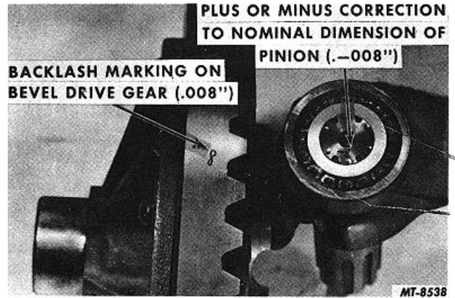
Fig. 25 Location of Pinion Setting Markings
