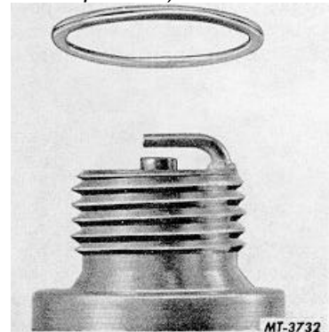
Fig. 2 Overtightened (Gasket Distorted)
