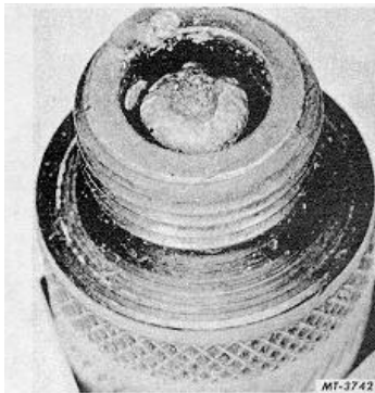
Fig. 12 Sustained Preignition Damage
