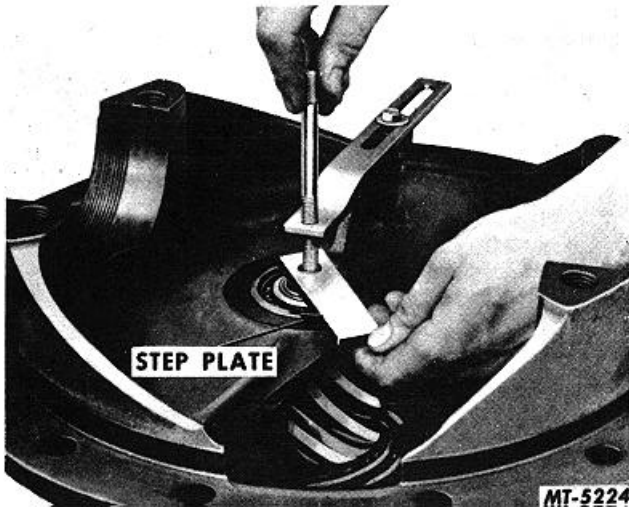
Fig. 27 Installing Step Plate
