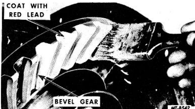
Fig. 32 Painting Gear Teeth for Obtaining Tooth Contact Impressions
