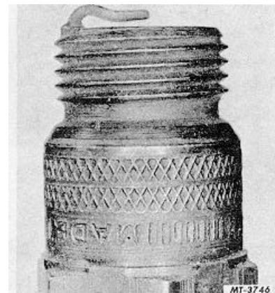
Fig. 16 Damage to Spark Plug from Pressure (Plier) Type Gap Tools
