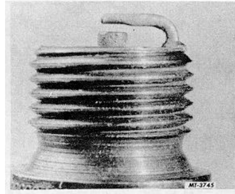
Fig. 15 Reversed Coil Polarity
