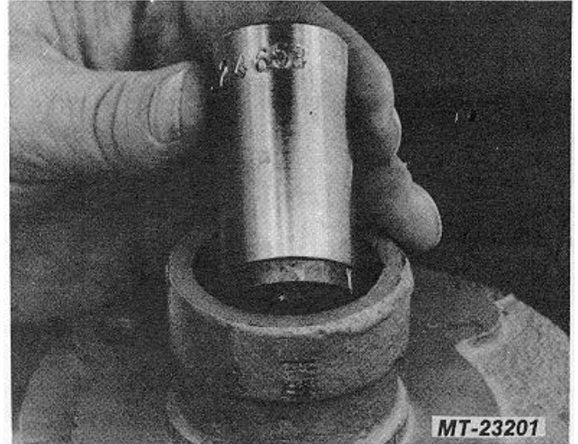
Fig. 22 Install New Pump Seal
